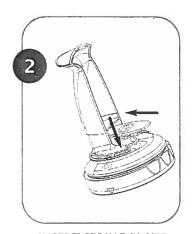
INSERT SPRING PLATE INTO THE HANDLE
