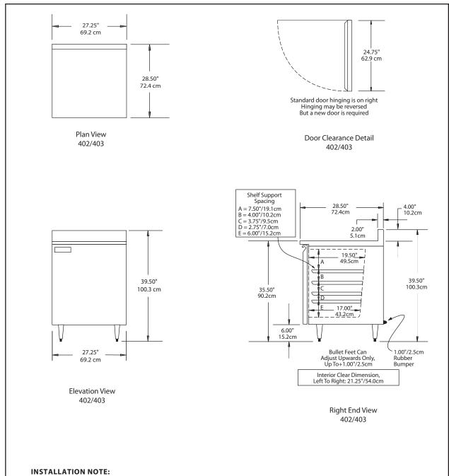
Refrigeration system is designed so that air will flow under the unit, through the compressor area and out the top rear of the unit. Any restriction to this air flow path will void the warranties.
